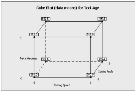
A. When the cutting speed increased from low to high level, the tool age increases
