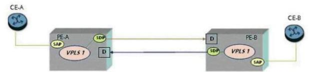
Assume the port on CE-A is sending two tags, a top tag of 100 and a bottom tag of 500. PE-A is configured with a SAP id of 1/1/1:100.\*. How should PE-B be configured if CE-B is expecting a top tag of 200 and a bottom tag of 500?
