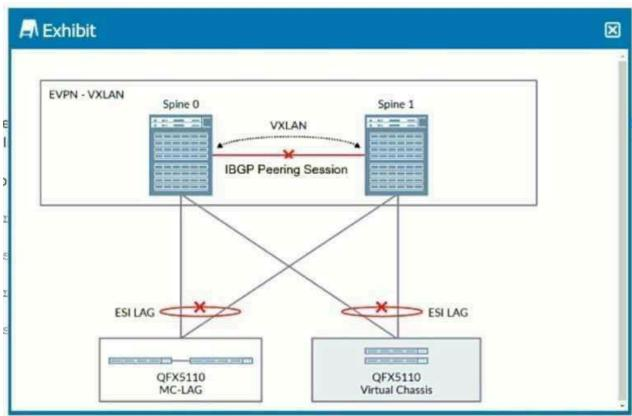
you have a data center in which only the spine devices are using EVPN and VXLAN. The leaf nodes are multihomed in active-active mode to the spine nodes through ESI LAG interfaces. In this design, a link failure on the interface connecting the spine nodes would also cause all traffic from the spine to the leaf nodes to drop.
